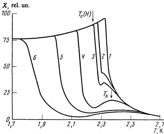
FIG. 1. Temperature dependences of the magnetic susceptibility of CuRb<sub>2</sub>Br<sub>4</sub> · 2H<sub>2</sub>O in the difficult magnetization direction at a pressure 9.5 kbar in dc magnetic fields: 1— $H = 0$ ; 2— $H = 50$  Oe; 3— $H = 70$  Oe; 4— $H = 110$  Oe; 5— $H = 200$  Oe; 6— $H = 250$  Oe.
