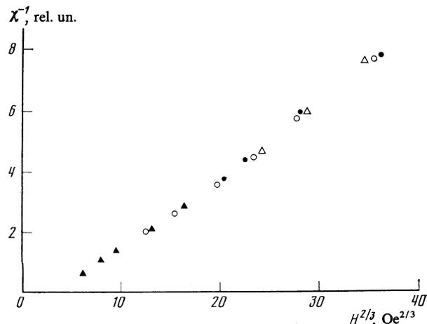
FIG. 3. Change of  $\chi_{\perp}^{-1}(T_h)$  in a magnetic field at fixed pressures [kbar]:  $\blacktriangle$ — $P = 0$ ;  $\circ$ — $P = 0$ ;  $\triangle$ — $P = 5.2$ ;  $\bullet$ — $P = 9.5$ .
