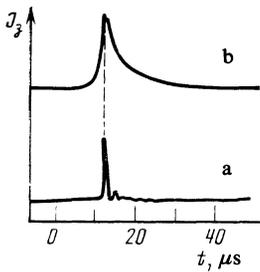
FIG. 5. Oscilloscope traces of the signals from the antenna (a) and from the double probe (b).
