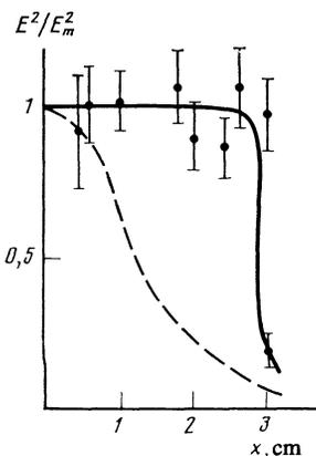
FIG. 6. Transverse field distribution in the focal region measured in the presence of the plasma (solid line) and in the absence of the plasma (dashed line).
