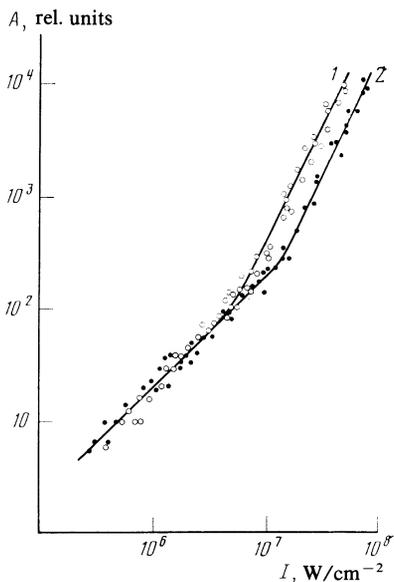
FIG. 4. Amplitude  $A(I)$  of the acoustic signal for the following specimens ( $\lambda = 0.27 \mu\text{m}$ ): 1—KBr ( $\alpha = 0.07 \text{ cm}^{-1}$ ) and 2—KCl ( $\alpha = 0.08 \text{ cm}^{-1}$ ).
