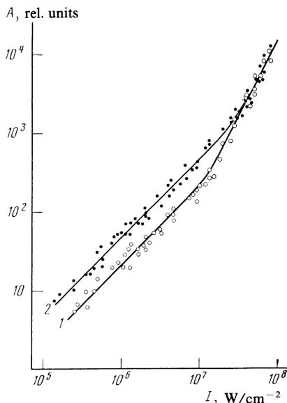
FIG. 3. Amplitude  $A(I)$  of the acoustic signal for two specimens of KCl with different linear absorption coefficients ( $\lambda = 0.27 \mu\text{m}$ : 1— $\alpha = 0.08 \text{ cm}^{-1}$ , 2— $0.24 \text{ cm}^{-1}$ ).
