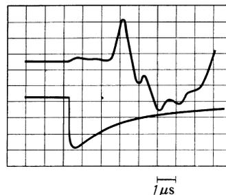
FIG. 1. Oscillogram of the acoustic signal (the lower trace is the laser pulse).
