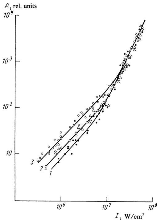
FIG. 2. Amplitude  $A(I)$  of the acoustic signal for three specimens of KBr with different linear absorption coefficients ( $\lambda = 0.35 \mu\text{m}$ : 1— $\alpha = 0.04 \text{ cm}^{-1}$ , 2— $0.07 \text{ cm}^{-1}$ , 3— $0.12 \text{ cm}^{-1}$ ).
