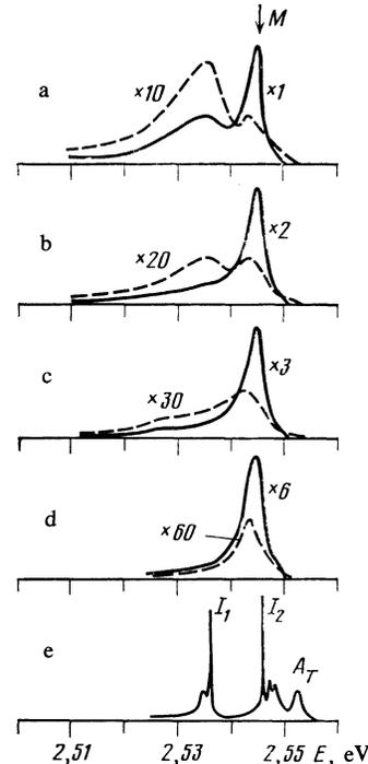
FIG. 1. Recombination-radiation spectra of CdS crystal in the polarizations  $E \perp c$  (solid curves) and  $E \parallel c$  (dashed curves) at various optical-pumping levels in  $\text{MW}/\text{cm}^2$ : a) 12, b) 5.5, c) 3, d) 1.4, e) excitation with mercury lamp. Crystal thickness  $d = 4.5 \mu\text{m}$ , temperature in thermostat 4.5 K, excitation-spot diameter  $\leq 10 \mu\text{m}$ .
