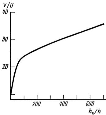
FIG. 4. Dependence of the voltage drop across the sample on the external magnetic field for  $I/i = 100$ .
