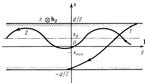
FIG. 1. The coordinate system; trajectories of the drifting (1) and trapped (2) electrons in the metal plate.
