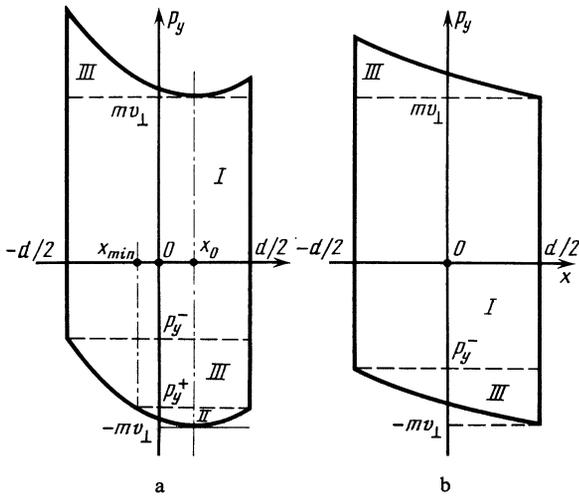
FIG. 2. The  $(x, p_y)$  phase plane and the regions of existence of the various electron groups in a) a sign-variable ( $h_0 < H$ ) resultant magnetic field and b) a resultant magnetic field of constant sign ( $H < h_0$ ): I) the region of existence of the untrapped electrons, II) that of the trapped electrons, and III) that of the surface electrons.
