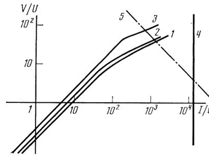
FIG. 3. The current-voltage characteristic, depicted on a double logarithmic scale, of a metallic plate for different values of the parameter  $h_0/h$ : the curve 1 corresponds to  $h_0/h < 1$ ; the curve 2, to  $h_0/h = 10$ ; the curve 3, to  $h_0/h = 100$ . On the vertical straight line 4 the radius  $R = 10^{-3}$  cm and the dot-dash straight line 5 corresponds to  $IV/LD = 1$  W/cm<sup>2</sup> ( $i = 0.86$  A and  $U = 3.1 \times 10^{-3}$  V).
