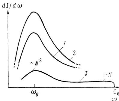
FIG. 3. Spectral density of radiation by channeled particles. 1) crystal without defects; 2) crystal with point defects; 3) difference of curves 2 and 1.  $N$  is the number of collisions of particles with defects.
