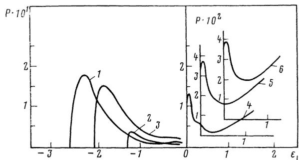
FIG. 4. Probability of dechanneling of 20 Mev electrons (1–3) and positrons (4–6) at point defects in a silicon crystal ( $\langle 110 \rangle$  axis). 1)  $x_g = 1$ ,  $Z_g = 14$ ; 2)  $x_g = 2$ ,  $Z_g = 14$ ; 3)  $x_g = 1.4$ ,  $Z_g = 83$ ; 4)  $x_g = 11$ ,  $Z_g = 14$ ; 5)  $x_g = 9$ ,  $Z_g = 70$ ; 6)  $x_g = 8$ ,  $Z_g = 81$ . The transverse energy is expressed in units of the critical Lindhard energy.
