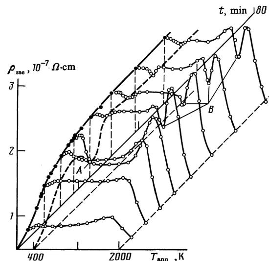
FIG. 3. The dependence of magnetoresistance  $\rho_{\text{sse}}$  of a specimen on annealing temperature  $T_{\text{ann}}$  for different times  $t$  for adsorption of oxygen on the surface,  $H = 10$  kOe,  $J \parallel [100]$ , H1J, H1n.
