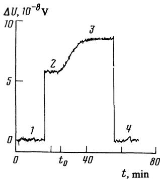
FIG. 1. Automatic trace of the dependence of the signal  $\Delta U$  from the potential contacts of a thin single-crystal plate of tungsten on time  $t$  in the absence of a magnetic field,  $n \perp (110)$ ,  $J \parallel [100]$ ,  $T = 4.2$  K. Sections 1 and 4 correspond to the trace when the current through the specimen is switched off, sections 2 and 3 to the measuring current  $J$  being switched on. The oxygen source is connected at the instant  $t_0$ .
