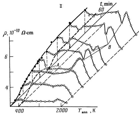
FIG. 2. The dependence of the resistivity  $\rho$  of a tungsten plate on annealing temperature  $T_{\text{ann}}$  for different times  $t$  for adsorption of oxygen on the surface of the specimen.
