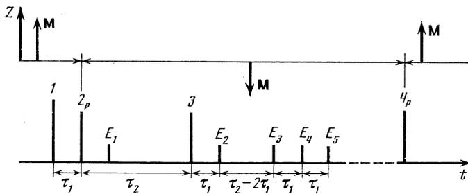
Fig. 2. Time sequence of pulses and signals: 1 and 3—high frequency pulses,  $2_p$ —pulse initiating rapid magnetic reversal,  $4_p$ —auxiliary magnetization-reversing pulse,  $E_1$ – $E_5$ —echo signals.
