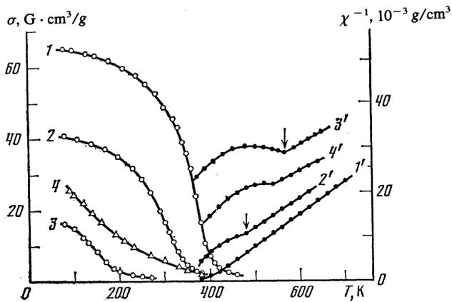
FIG. 5. Temperature dependence of specific magnetization and inverse susceptibility,  $\chi^{-1}$  (curves denoted by primed numbers) for the  $\text{Mn}_{1-x}\text{Cr}_x\text{Sb}$  alloys measured in a field of 8 kOe for the annealed alloys: 1 and 1')  $x = 0.5$ ; 2 and 2')  $x = 0.6$ ; 3 and 3')  $x = 0.75$ ; and for the quenched alloy: 4 and 4')  $x = 0.7$ . The arrows indicate  $T_N$ .
