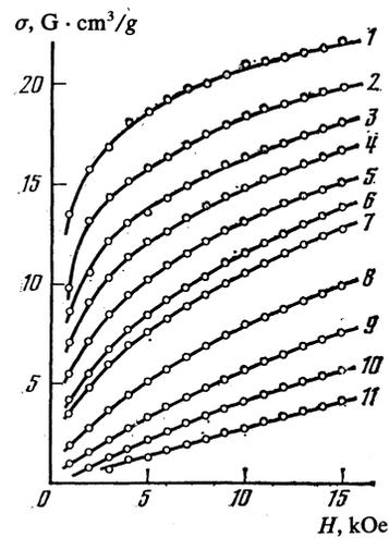
FIG. 3. Magnetization curves of  $Mn_{0.4}Cr_{0.6}Sb$  in the vicinity of the canted-ferromagnetic-antiferromagnetic transition. Temperatures in K are: 1) 290; 2) 298; 3) 303; 4) 308.3; 5) 313; 6) 318; 7) 323; 8) 333; 9) 343; 10) 353; and 11) 368.
