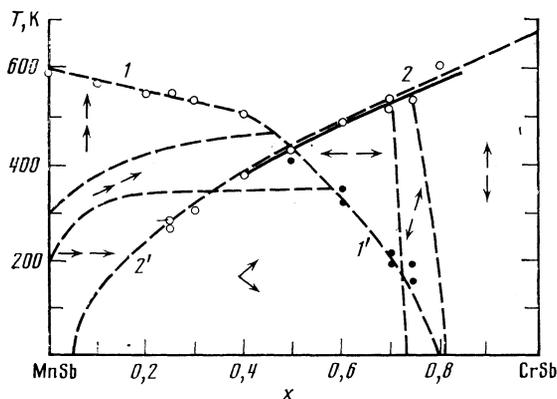
FIG. 2.  $Mn_{1-x}Cr_xSb$  magnetic phase diagram plotted from the temperature dependence of  $\Delta I/I$  (O) and from the magnetic measurements (●). The solid curve corresponds to first-order phase transitions, the dashed curves to second-order phase transitions.<sup>6</sup>
