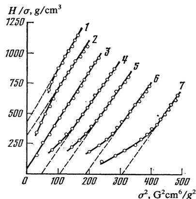
FIG. 4. Dependence of the ratio  $H/\sigma$  on  $\sigma^2$  for  $Mn_{0.4}Cr_{0.6}Sb$  in the vicinity of the canted-ferromagnetic-antiferromagnetic transition. Temperatures in K are: 1) 323; 2) 318; 3) 313; 4) 308.3; 5) 303; 6) 298; and 7) 290.
