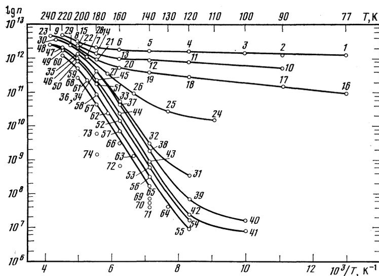
FIG. 4. Temperature dependences of the electron density in the conduction band for the second sample. The dependences were plotted in a time interval ( $\sim 9$  h) near the conversion.
