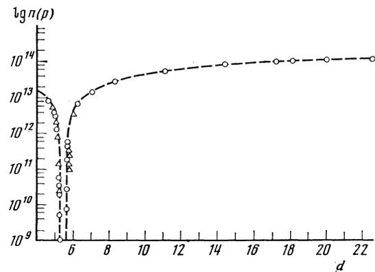
FIG. 2. Electron (hole) density in band vs. time after irradiation.  $\circ$ —1st sample,  $\triangle$ —2nd sample, dashed line—calculated curve; left- and right-hand branches—electron and hole densities, respectively.
