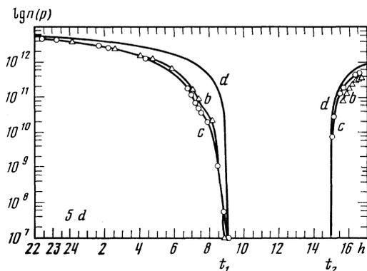
FIG. 3. Time dependence of the electron (hole) density in the band near the conversion instant, *c*, *b*—experimental curves for 1st and 2nd samples, respectively, *d*—calculated curve. Left- and right-hand branches—electron and hole densities, respectively.
