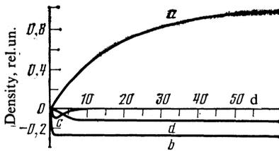
FIG. 1. Calculated time dependences of the densities of the electrically active centers that result from irradiation by thermal neutrons:  $a - \text{Ga}^{71}$ ;  $b - \text{As}^{75}$ ;  $c - \text{As}^{77}$ ;  $d - \text{Se}^{77}$ . The final (asymptotic)  $\text{Ga}^{71}$  density is taken to be unity. The scales of the  $\text{As}^{77}$  and  $\text{Se}^{77}$  plots are magnified 10 times.
