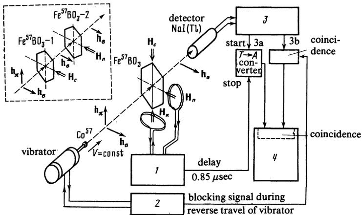
FIG. 1. Schematic diagram of apparatus for studying modulation of  $Fe^{57}$  Mössbauer radiation. 1) magnetization pulse generator, 2) vibrator control, 3) fast and slow amplifier and discriminator (3a is the fast channel; 3b is the slow channel), 4) NTA-512 multichannel analyzer. The insert depicts the final modulation scheme.
