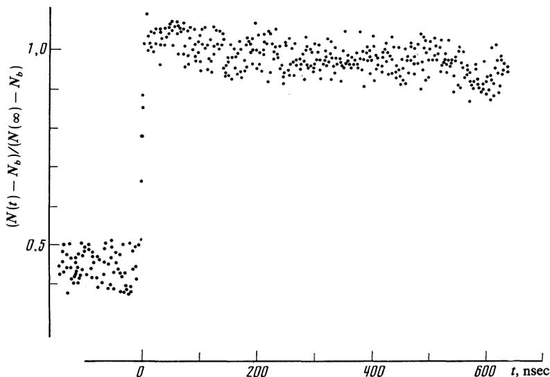
FIG. 3. Time dependence of  $\text{Fe}^{57}$   $\gamma$  ray intensity obtained in the final modulation scheme.  $N_b$  is the nonresonance background, (1 channel = 1.8 nsec).
