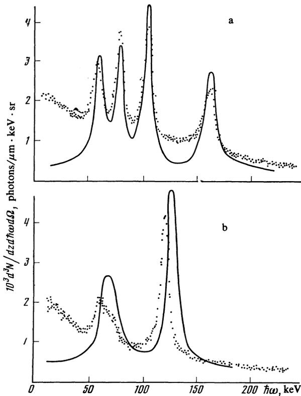
FIG. 2. Emission spectrum of 54-MeV electrons in diamond: a) the (110) plane; b) the (100) plane; the points are the experimental results of Ref. 19, the curves are theoretical.
