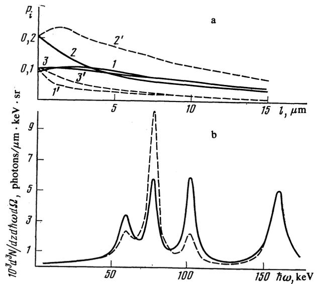
FIG. 3. a) The influence of laser radiation on the kinetics of the band populations; curves 1, 2, and 3 correspond to bands 3, 4, and 5; b) the change in the spectrum. The solid and dashed curves are for the cases with and without laser radiation, respectively. C(110),  $E = 54$  MeV.
