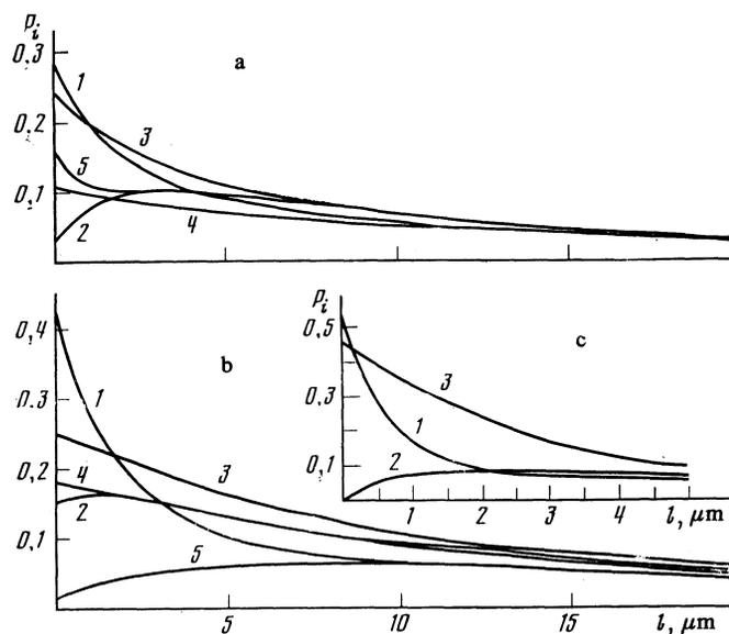
FIG. 1. Kinetics of band populations in terms of the depth of penetration of the particle into the crystal: a) C(110), with six bands in the potential well; b) C(100), with three bands,  $E = 54$  MeV; the curves are labeled with the numbers of the bands; c) Si(110),  $E = 4$  MeV; curves 1 and 2 are levels inside the potential well, curve 3 is an above-barrier level.
