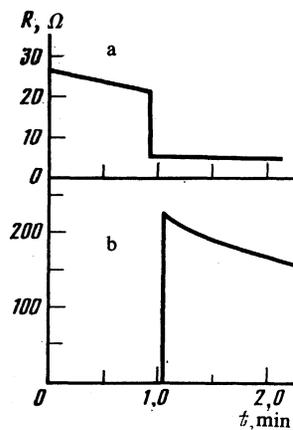
FIG. 1. Change of the resistance in the course of condensation of Yb and Bi films on substrates cooled with liquid helium: a—Yb film,  $D_{cr} = 110$  nm, condensation rate  $v_{cond} \approx 60$  nm/min; b—Bi film,  $D_{cr} \approx 36$  nm,  $v_{cond} \approx 10$  nm/min.
