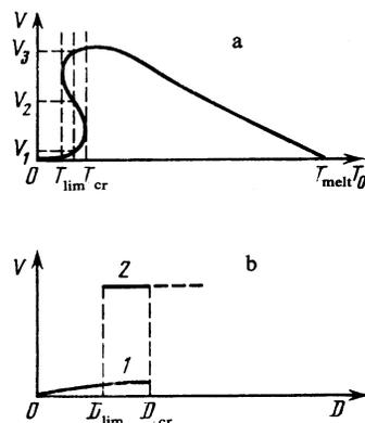
FIG. 6. Schematic plots of the crystallization front velocity vs the substrate temperature (a) and the film thickness (b).
