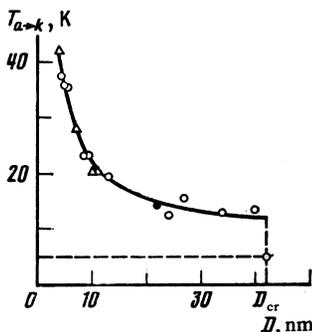
FIG. 5. Dependence of crystallization temperature of amorphous Bi films on their thickness  $\circ$ —for  $T_0 = 4.2$  K;  $\triangle$ — $T_0 = 20.4$  K;  $\bullet$ — $T_0 = 14.3$  K. The horizontal dashed line corresponds to the average film temperature  $T'_0$  in the course of their condensation; the vertical dashed line corresponds to the critical thickness (both lines are for  $T_0 = 4.2$  K).
