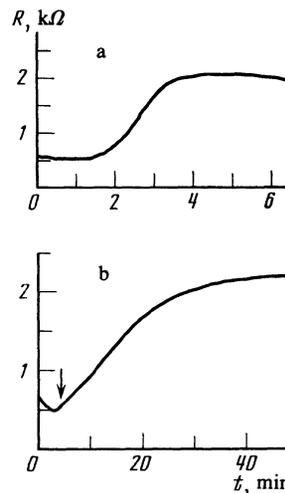
FIG. 4. Time dependence of resistance of Bi film condensed at  $T_0 = 20.4$  K: a—in the course of continuous condensation; final film thickness  $D \approx 21$  nm,  $v_{cond} \approx 1.5$  nm/min; b—with the film maintained at  $T_0 = 20.4$  K. The arrow shows the instant when condensation stops at  $D \approx D_{a \rightarrow k} \approx 10$  nm.
