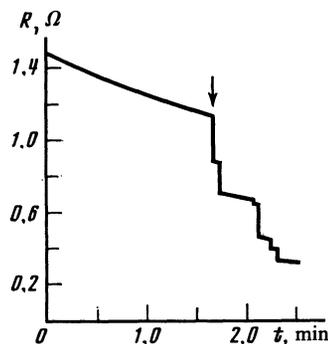
FIG. 3. Variation of resistance during the time of condensation of a Ga film on a substrate cooled with liquid helium. The arrow shows the instant when the film reaches critical thickness.  $D_{cr} \approx 210$  nm;  $v_{cond} \approx 33$  nm/min.
