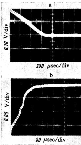
FIG. 2. Oscillograms of spontaneous crystallization of amorphous Yb (a) and Bi (b) films when they reach critical thickness in the course of condensation. The inclined sections of the oscillograms correspond to the vertical sections of the corresponding curves in Fig. 1.
