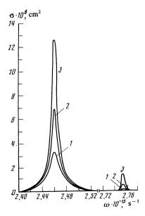
FIG. 1. Extinction cross section of small particles of potassium localized in a KCl crystal as a function of the frequency of incident radiation, without taking into account nondissipative damping (Q < 1, Ref. 2), for three values of the particle size  $1 - a = 5.2 \times 10^{-6}$  cm;  $2 - a = 6.2 \times 10^{-6}$  cm  $3 - a = 7.2 \times 10^{-6}$  cm.
