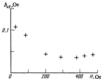
FIG. 1. Dependence of the threshold field  $h_{c2}$  on the strength of the static field  $\mathbf{H}$  perpendicular to the binary axis, at  $T = 2.2$  K.
