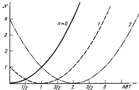
FIG. 2. Dependence of the kinetic energy of superfluid flow on the temperature difference  $\delta T$  at  $n = 0, 1$ , and 2.
