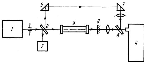
FIG. 1. Diagram of experimental setup. 1—dye laser, 2—laser-energy meter, 3—cell with potassium and buffer gas, 4—DFS-8 spectrograph, 5, 8—mirrors ( $R = 50\%$ ), 6, 7—prisms, 9—mirror ( $R = 100\%$ ).
