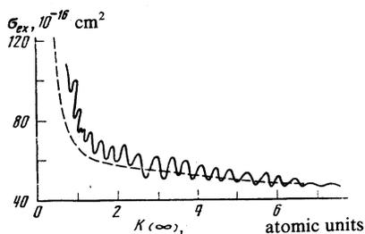
FIG. 2. Cross section for the resonant charge-exchange reaction  $p + H \rightarrow H + p$  as a function of the relative momentum  $K(\infty)$ . The solid line shows the result of Ref. 15, and the dashed line is the result of the present work.
