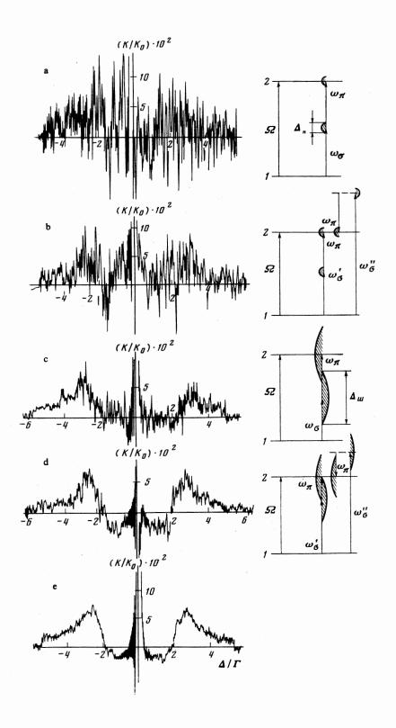
FIG. 5. Absorption spectra of weak sounding monochromatic radiation (nonlinear interference effect) for different widths of the noise-pump spectrum and different two-photon excitation mechanisms: a, b ( $\Delta_n = 300 \text{ Hz}$ ) and c, d ( $\Delta_n = 3 \text{ kHz}$ )—noise pumping, e—monochromatic pumping. The shaded sections show the width  $\Delta_n$  of the noise-field spectrum;  $\Delta = \Omega - \omega_{21}$ .
