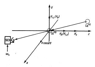
FIG. 2. Optical orientations of the  $Cd^{113}$  atoms. SD—synchronous detector.
