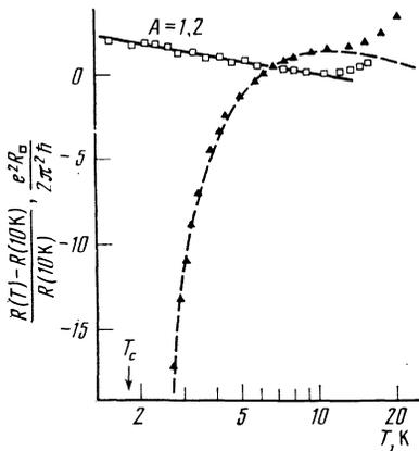
FIG. 7. Plot of  $R(T)$  obtained for Al 1 at  $H=0$  ( $\blacktriangle$ ) and  $H=30$  kOe ( $\square$ ). Dashed line—theoretical plot of Eq. (1).
