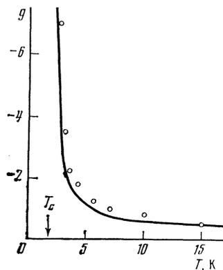
FIG. 6. Plot of  $g(T)$  for sample Nb 2. Solid line—theoretical plot of  $g(T)$ .
