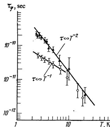
FIG. 3. Plots of  $\tau_{\varphi}(T)$  for aluminum samples:  $\blacktriangle$  - Al 1,  $\circ$  - Al 2.
