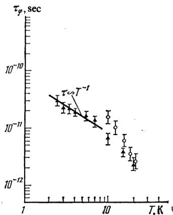
FIG. 4. Plots of  $\tau_\varphi(T)$  for niobium samples:  $\circ$  — Nb 1,  $\blacktriangle$  — Nb 2.
