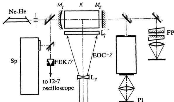
FIG. 1. Experimental setup,  $K$ —cell with carbon disulfide,  $M_1$  and  $M_2$ —dielectric mirrors,  $L_1$  and  $L_2$ —dielectric lenses, FP—Fabry-Perot interferometer, Sp—prism spectrograph, EOC—electron-optical camera.
