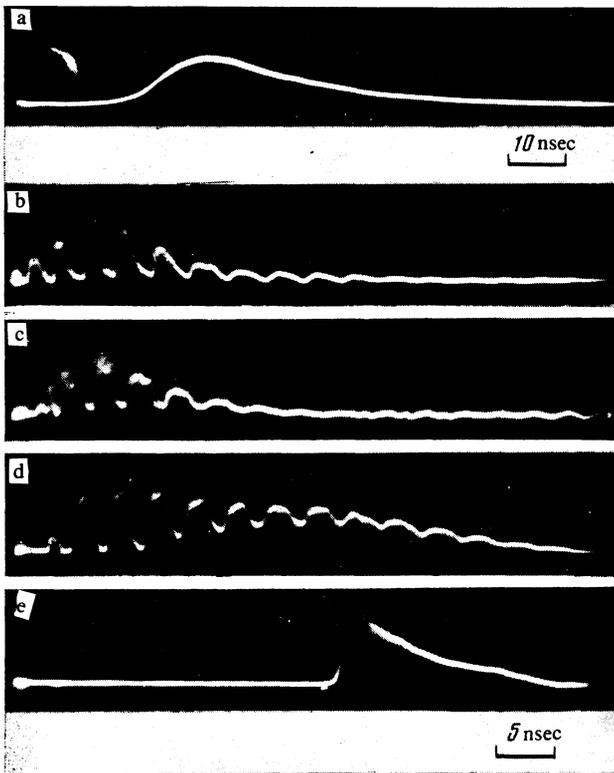
FIG. 3. Oscillograms of the pump radiation (a) as well as of the SRS radiation (b-d) and of the SRS (e) excited in the external cavity.
