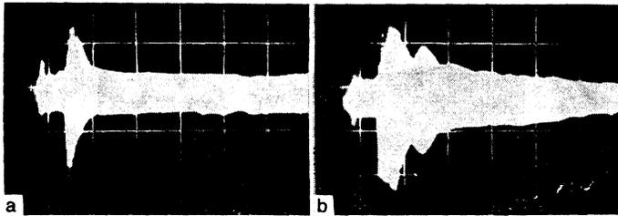
FIG. 4. Oscilloscope of microwave power passing through the resonator close to the instant of time when a mechanical shock is produced in the sample ( $H = 0.4$  kOe, sweep  $100 \mu\text{sec}/\text{div}$ ): a)  $h/h_e = 0.15$ ; b)  $h/h_e = 0.9$ .
