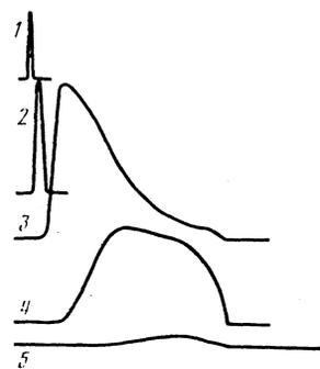
FIG. 6. Plot of signal of the piezo-sensor as a function of the magnetic field. Width of passband of the tuned amplifier 0.01 MHz. The tuned amplifier is tuned to the frequency (in MHz): 1) 2.42; 2) 2.43; 3) 2.45; 4) 2.46; 5) 2.47; ( $\pm 0.01$ ).
