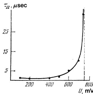
FIG. 10. Lifetime of collective oscillations of frequency  $\Omega = 1.23$  MHz vs amplitude of ac voltage of frequency  $2\Omega$  on the piezosensor.
