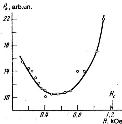
FIG. 5. Dependence of the threshold generation power of 2.4-MHz elastic oscillations on the magnetic field.
