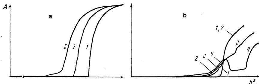
FIG. 9. Dependence of the piezo-sensor signal amplitude at 2.4 MHz on the power of the first pump under the action of the second pump. a)  $\Delta f = (\omega_{p2} - \omega_{p1})/2\pi > 0$ : 1) generator  $G_2$  turned off; 2)  $h_2/h_{2c} \approx 2$  and  $\Delta f = 4.5$  MHz; 3)  $h_2/h_{2c} \approx 2$  and  $\Delta f = 4.8$  MHz; b)  $\Delta f = -4.8$  MHz; 1) generator  $G_2$  turned off; 2)  $h_2 = h_{2c}/4$ ; 3)  $h_2 = 1.2h_{2c}$ ; 4)  $h_2 \approx 2h_{2c}$ .
