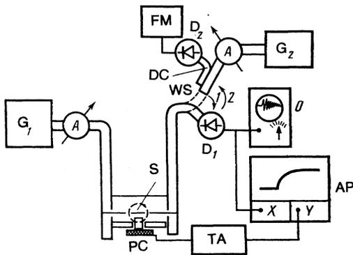
FIG. 1. Experimental setup:  $G_1, G_2$ ) microwave generators; A) attenuators; DC) directional coupler; WS) waveguide switch; PC) piezoceramic; S) Strip of strip resonator (the dashed lines show the direction of the microwave magnetic field);  $D_1, D_2$ ) microwave detectors; FM) frequency meter; O) oscilloscope; AP) automatic plotter; TA) tuned amplifier.
