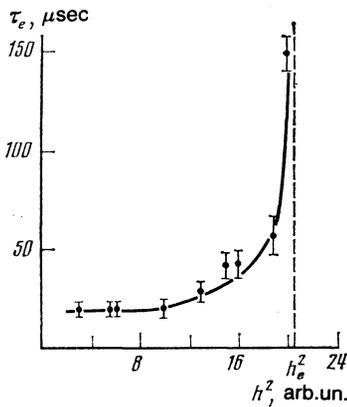
FIG. 7. Dependence of the lifetime of the elastic oscillations of the 2.4-MHz mode on the microwave pump power.
