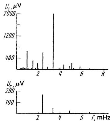
FIG. 3. Spectrum of the oscillations of the microwave power passing through the resonator ( $U_1$ ) and of the piezoceramic signal  $U_e$  at  $h/h_c \approx 15$  and  $H = 0.4$  kOe.
