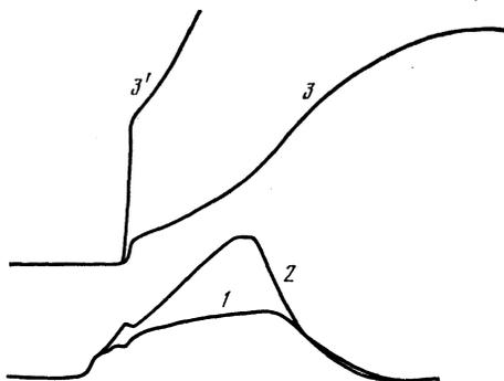
FIG. 2. Plot of piezo-sensor signal as a function of the microwave pump power (signal of detector  $D_1$ ). The tuned amplifier with passband 0.01 MHz is tuned to the frequency (in MHz); 1) 2.38; 2) 2.40; 3) 3.32;  $H = 0.4$  kOe. The plot of line 3' was obtained at a higher sensitivity of the amplifier.
