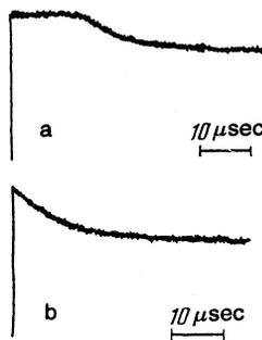
FIG. 8. Envelope of detector signal  $D_2$  when SW + waves are observed: a)  $h < h_e$ ; b)  $h > h_e$ .
