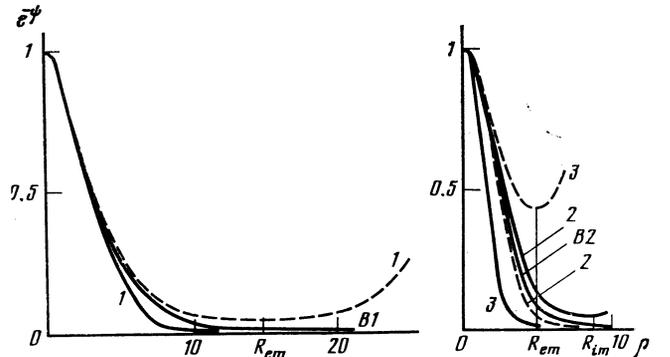
FIG. 1. Radial distribution of the particle density  $n/n_0 = e^{-\psi}$ . The curves are numbered in accord with the table. Electrons—dashed line, ions—solid. Curves  $B1$  and  $B2$  are Bennett distributions with respective parameters  $\beta_0^2 = 0.4, f_0 = 0.9, \tau_0 = 3$  and  $\beta_0^2 = 0.8, f_0 = 0.68, \tau_0 = 1.5$ .
