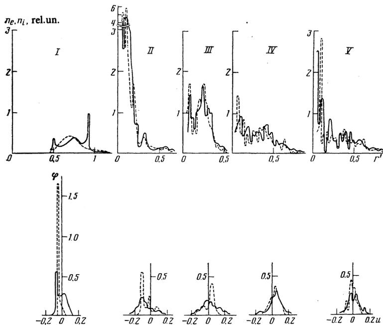
FIG. 3. Spatial evolution of radial dependences of the densities  $n_e$  and  $n_i$ , and of the particle distribution function  $\varphi$  averaged over the cross section, with respect to the radial velocities  $u = \sqrt{2}v_r/\omega_e r_0$  for different  $z$ : I— $z=5$ , II—15, III—19, IV—23, V—27;  $K=250$ . Solid lines—electrons, dashed—ions.
