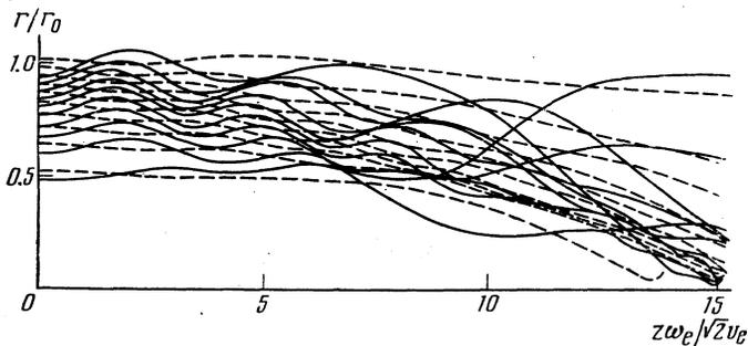
FIG. 2. Particle trajectories in superimposed cold beams. Solid lines—electrons, dashed—ions.
