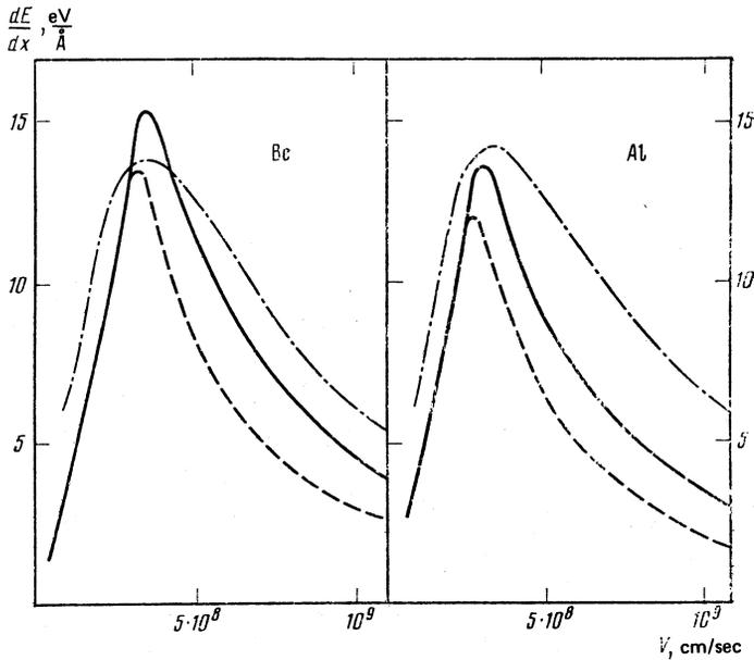
FIG. 3. Proton energy losses in beryllium and aluminum. The dash-dot curves are plots of the interpolation formulas given in Ref. 15 and agree well with the experimental results. Solid lines—theoretical calculation, dashed—calculation without allowance for plasmon excitation. The electron effective mass is assumed equal to the free-electron mass.
