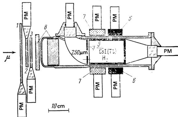
FIG. 2. Diagram of experimental setup: 1) counter that monitors the passage of the second meson; 2, 3, 4) monitoring counters; 5) vessel counter enclosing the working volume of the target; 6, 7) secondary-particle detectors with NaI and stilbene scintillators, respectively; 8) decelerating filter; PM) photomultiplier.
