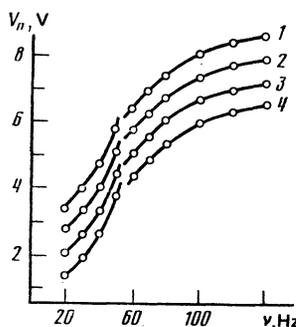
FIG. 1. Dependence of the threshold voltage on the frequency at different sample thicknesses: 90  $\mu\text{m}$  (1); 60  $\mu\text{m}$  (2); 30  $\mu\text{m}$  (3); extrapolation to "zero" thickness (4) (120 °C).
