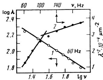
FIG. 3. Dependence of the period of the domains on the frequency in different coordinate axes:  $\log \lambda$  ( $\log \nu$ )—1;  $\lambda^{-2}(\nu)$ —2; (120 °C, 30  $\mu\text{m}$ ).
