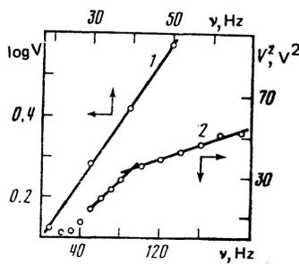
FIG. 2. Threshold voltage  $V(v,0)$  plotted in different coordinates:  $\log V(v)$ —1,  $V^2(v)$ —2.
