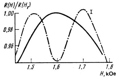
FIG. 4. Shape of GMR curve in the region of the proposed fine structure. Solid line—experimental data for N<sub>2</sub> at  $p = 30$  mTorr,  $H_1 = 180$  Oe,  $f = 338$  kHz. Dash-dot line—theoretical curve. On the upper right is shown the mean-squared error bar.
