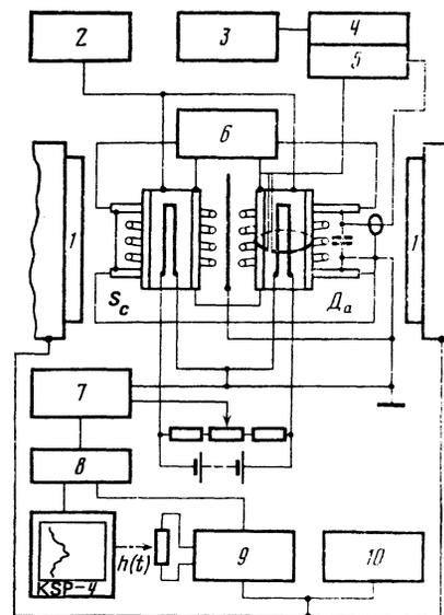
FIG. 1. Block diagram of the experimental setup: 1—electromagnet; 2—system for evacuation and filling; 3—master oscillator Ch6-31; 4—power amplifier; 5—amplitude stabilizer; 6—thermal stabilization system; 7—F116/1 amplifier; 8—synchronous detector; 9—modulator; 10—stabilizer for the field  $H_0$ ;  $S_c, S_a$ —comparison and active sensors.
