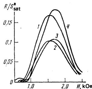
FIG. 3. Experimental curves of GMR in  $\text{N}_2$  (1,2) and  $\text{CO}$  (3,4) at  $p = 30$  mTorr,  $H_1 = 180$  Oe,  $f = 338$  kHz, and at two orientations of the temperature gradient  $\nabla T$  relative to  $\mathbf{H}$ : 1,4  $-\nabla T \parallel \mathbf{H}$ ; 2,3  $-\nabla T \perp \mathbf{H}$ .
