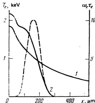
FIG. 5. Transverse profiles of  $T_e$  and  $|\omega_e \tau_e|$  at  $b = 33 \mu\text{m}$ ,  $q_0 = 4.5 \times 10^{14} \text{ W/cm}^2$ , and  $t = 0.3 \text{ nsec}$  near the critical surface. The dashed line is the profile of  $|\omega_e \tau_e|$ . Curves 1 and 2 correspond to calculations without and with generation of magnetic fields.
