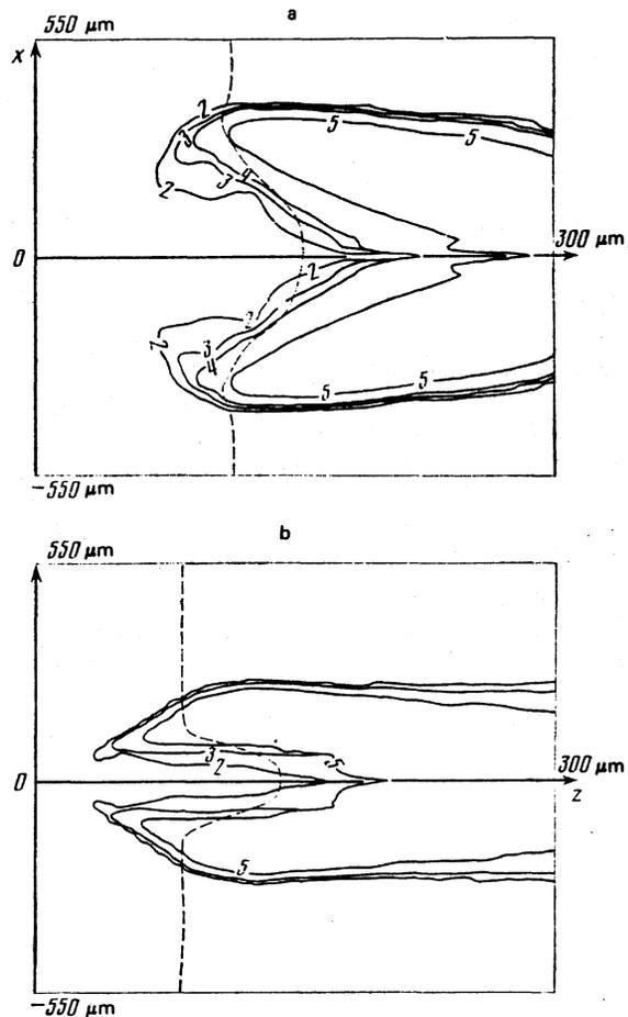
FIG. 2. Level lines of  $|\omega_e \tau_e|$  ( $t = 0.3$  nsec). Case a and b correspond to  $b = 200$  and  $33$   $\mu\text{m}$  and to  $q_0 = 0.75 \times 10^{14}$  and  $4.5 \times 10^{14}$   $\text{W}/\text{cm}^2$ , respectively. The line  $n_e = n_{ec}$  is shown dashed. Curve 2 corresponds to  $\omega_e \tau_e = 0.05$ , 3—0.4, 4—0.2, 5—0.5.
