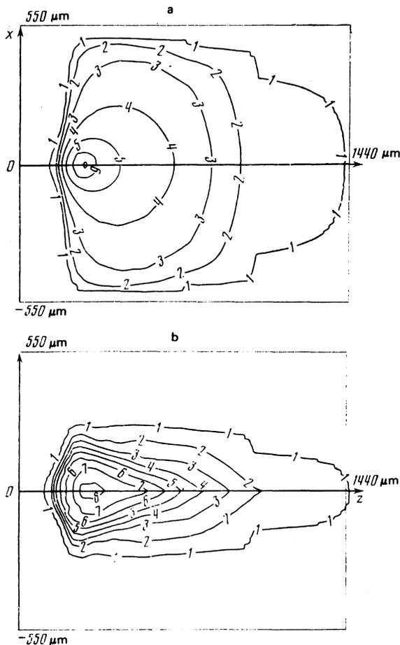
FIG. 4. Level lines of electron temperature at  $b = 33 \mu\text{m}$ ,  $q_0 = 4.5 \times 10^{14} \text{ W/cm}^2$ , and  $t = 0.3 \text{ nsec}$ . The case *a* pertains to the calculation without allowance for the generation and magnetic field, and case *b* to the complete formulation. The curve with index 1 corresponds to  $T_e = 0.025$ , 2—0.3, 3—0.6, 4—0.9, 5—1.2, 6—1.5, 7—1.8, and 8—2.1 keV.
