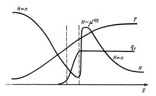
FIG. 4. Structure of the radiative cooling wave: T—plasma temperature, H—magnetic field,  $q_T$ —heat flux. The dashed lines mark the region that makes the principal contribution to the energy lost to radiation.
