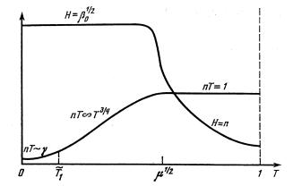
FIG. 3. Profiles of plasma pressure nT and of the magnetic field H in the case of an ideally conducting boundary at  $\beta_0 > \mu^{-1}$  and  $\delta_0 > \mu^{-3/4}$ .
