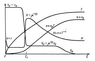
FIG. 2. Profiles of the temperature T, of the magnetic field H, of the plasma velocity v, and of the velocity of the thermal drift of the magnetic field  $V_H$  in the case of a nonconducting boundary at  $\beta_0 > \mu^{-1}$  and  $\delta_0 > \mu^{-3/4}$  (nT = 1).
