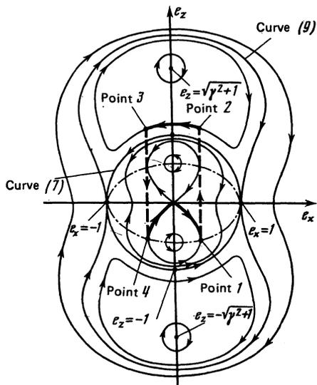
FIG. 1. Phase plane of the alternating components  $e_x$  and  $e_z$  of the electric field of a nonlinear TM wave. In the absence of the wave the plasma is supercritical ( $\epsilon_0 < 0$ ) and the nonlinearity is of the striction type ( $\delta = +1$ ). The thick (solid and dashed) lines single out a solution in the form of a waveguide channel of the simplest type.
