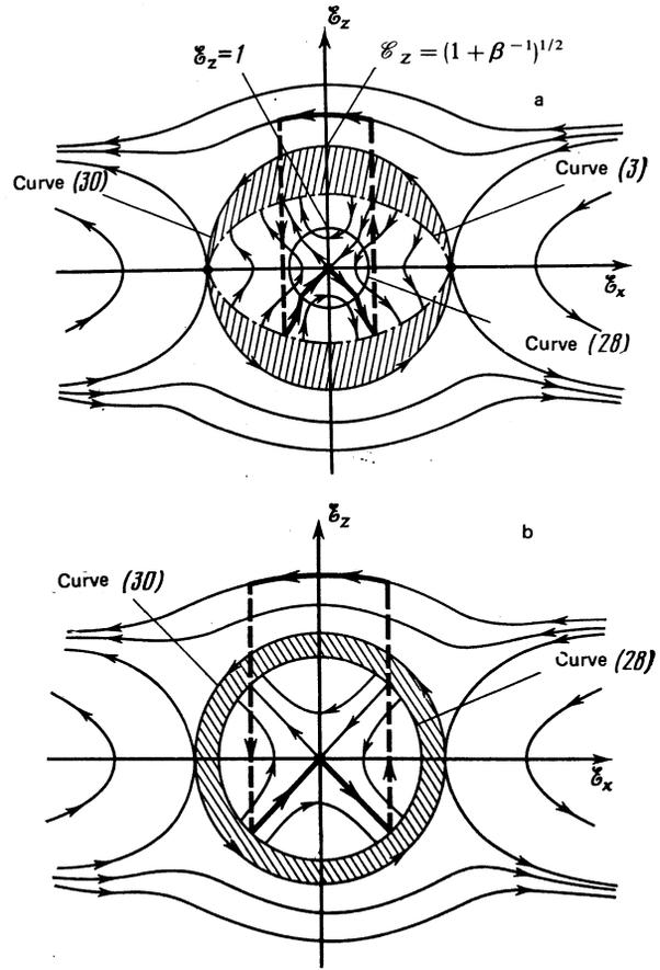
FIG. 3. Phase plane of the variables  $(\mathcal{E}_x, \mathcal{E}_z)$  for a plasma with ionization nonlinearity in the case of a nonzero threshold field  $E_a^2 > 0$  for different values of the parameter  $\beta$ : a)  $\beta < \beta^*$ , b)  $\beta > \beta^*$ . In the shaded region the behavior of the integral curves, which depends on the parameter  $\gamma^2$ , does not influence the plasma-waveguide solution outlined in the figure by a thick (solid and dashed) line.
