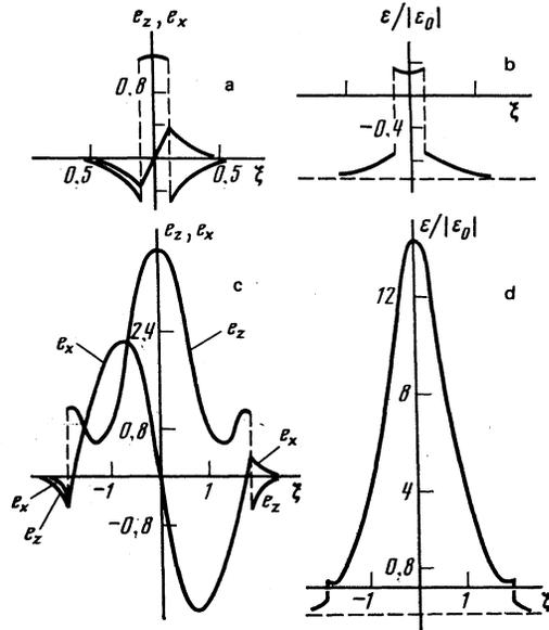
FIG. 2. Distributions of the field and of the dielectric constant in a self-sustaining waveguide channel for the first (a, b) and second (c, d) symmetric TM modes at  $\gamma = 3$ .
