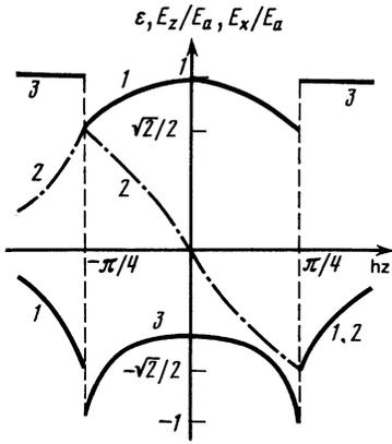
FIG. 4. Distribution of the electric-field components  $E_x$  (curve 1) and  $E_z$  (curve 2), and of the dielectric constant  $\varepsilon$  (curve 3) in a self-sustaining plasma waveguide in a medium with ionization nonlinearity at  $\gamma^2 \gg \beta > 1$ .
