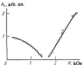
FIG. 2. Dependence of the threshold field  $h_c$  on the static field  $H$ ,  $T = 90$  K.
