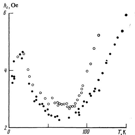
FIG. 3. Plots of  $h_c(T)$  at  $H < H_R$  and  $H > H_R$ ;  $\bullet$ — $H = 330$  Oe,  $\circ$ — $2.34$  kOe.
