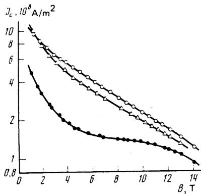
FIG. 2. Dependences of the critical-current density on the magnetic field at  $T = 4.2$  K for  $\text{PbMo}_6\text{S}_8$  samples with different grain size:  $\circ$ — $0.3 \pm 0.1$ ;  $\triangle$ — $0.7 \pm 0.2$ ;  $\bullet$ — $1.3 \pm 0.4$   $\mu\text{m}$ .
