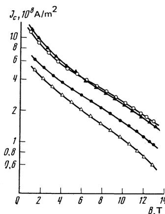
FIG. 1. Dependences of the critical-current density on the magnetic field at 4.2 K for one of the  $\text{PbMo}_6\text{S}_8$  samples after annealings at  $850^\circ\text{C}$  for 48 h:  $\Delta$ —first annealing;  $\bullet$ —second annealing;  $\blacktriangle$ —third annealing;  $\circ$ —fourth annealing.
