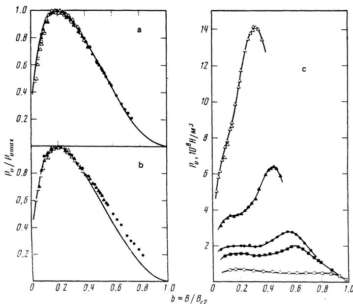
FIG. 3. Dependences of the pinning force on the relative induction at various temperatures:  $\circ$ — $2.4$  K;  $\triangle$ — $4.2$  K;  $\blacktriangle$ — $7.0$  K;  $\bullet$ — $8.5$  K;  $\blacksquare$ — $9.0$  K;  $\square$ — $10.5$  K for samples with grain size  $0.3 \pm 0.1$  (a),  $0.7 \pm 0.2$  (b), and  $1.3 \pm 0.4$   $\mu\text{m}$  (c).
