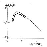
FIG. 6. Dependence of  $\Delta \rho / \rho$  on  $\tau_1^*$  at T = 1.4 K,  $\bullet$ —experimental points. The curves were calculated from Eq. (6); solid curves N = 8,  $W_c = 63$  sec<sup>-1</sup>, with account taken of  $\tau_1$ ; when account is taken of the exchange field  $H_{ee}$ , the same curve corresponds to N = 20, the dashed curve — N = 9,  $W_c = 63$  sec<sup>-1</sup>,  $\alpha = 10^{-5}$ .
