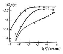
FIG. 4. Dependence of the SDR on the microwave power at T = 1.4 K;  $\Box - \rho = 3 \cdot 10^9 \, \Omega \cdot \text{cm}, f_M > (\tau_1^*)^{-1}; \circ - \rho = 5 \cdot 10^8 \, \Omega \cdot \text{cm}, f_M = 0;$  $\Delta - \rho = 5 \cdot 10^7 \, \Omega \cdot \text{cm}, \text{ and } f_M > (\tau_1^*)^{-1}$ . The solid curves were calculated from formula (6).
