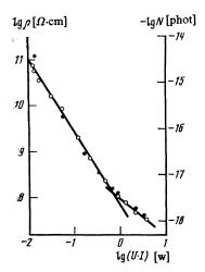
FIG. 9. Dependence of the resistance of the sample (O) and of the number of photons absorbed by the sample ( $\bullet$ ) on the lamp power at T = 1.4 K.
