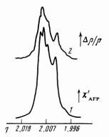
FIG. 1. DDB EPR spectrum,  $\chi'_{AFP}$ , and the SDR spectrum ( $H_1 = 0.02$ Oe) at T = 1.4 K;  $H_0 || [111]$ ;  $H_0 = 3.3$  kOe.
