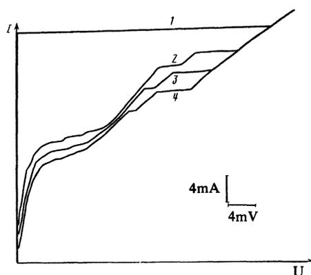
FIG. 9. Current-voltage characteristics of sample In-4 obtained for different values of the heater current  $I_h$  (mA): 1) 0; 2) 0.3; 3) 0.4; 4) 0.5. The results illustrate how to separate superdomains on the basis of the current.
