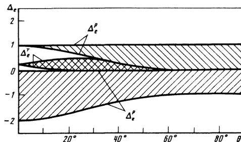
FIG. 3. Angular dependences of the boundaries  $\Delta_s^T$  and  $\Delta_s^b$  of the regions of selective reflection (the region of reflection of light of arbitrary polarization is shown cross hatched).
