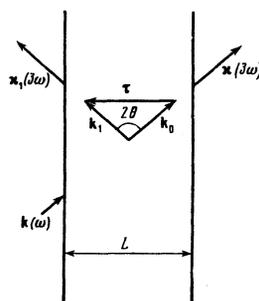
FIG. 1. Illustrating the geometry of frequency conversion under selective-scattering conditions.
