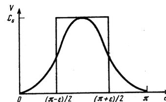
FIG. 4. Illustrating the replacement of the real interaction by a step.
