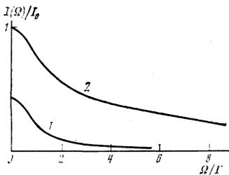
FIG. 6. Contour of spectral line in the limiting case of strongly anisotropic collisions ( $J=10$ ): 1) contour for transition with sublevel  $M = \pm J$ ; 2) summary contour.
