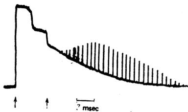
FIG. 6. Oscillogram, illustrating the method of determining  $T_n(t)$ , of the microwave power after it had passed through the resonant cavity.
