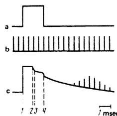
FIG. 2. Scheme of oscillograms: a) output power of  $G 1$ ; b) output power of  $G 2$ ; c) microwave power after it had passed through the resonant cavity.
