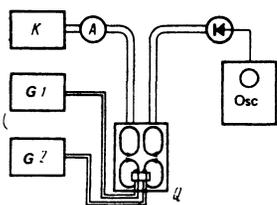
FIG. 1. Block diagram of the setup: K) klystron, A) precision attenuator, G1) and G2) rf oscillators, and Q) microwave resonant cavity.
