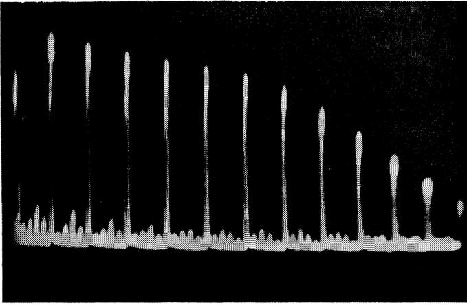
FIG. 2. Oscillogram of echoes of longitudinal hypersound in a sapphire crystal in the case of planar-spherical geometry of the reflecting surfaces. Every fifth echo is separated in amplitude.
