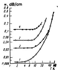
FIG. 3. Temperature dependence of the damping of longitudinal hypersound in lithium niobate along a threefold axis at a frequency of 3 GHz—(1) and (3), 9.4 GHz—(2) and (4); 1 and 2—with reversal ( $R = 44.8$  mm,  $L = 442$  mm,  $\epsilon = -0.2$ ), 3 and 4—without reversal.
