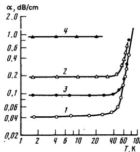
FIG. 4. Temperature dependence of the damping of longitudinal hypersound in sapphire along a threefold axis at a frequency of 3 GHz—(1) and (3), 9.4 GHz—(2) and (3); 1 and 2—with reversal ( $R = 44.8$  mm,  $L = 22.5$  mm,  $\epsilon = -0.016$ ), 2 and 4—without reversal.
