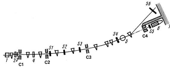
FIG. 1. Diagram of experiment. 1—pulsed magnet, 2—tungsten target, 3 and 4—secondary-emission monitors, 5—goniometer, 6—NaI(Tl) spectrometer, 7—lead shield, K1—K4—collimators,  $\nabla$ —deflecting magnets, S1—S6—scintillation counters.
