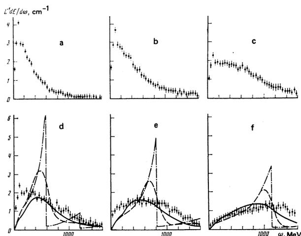
FIG. 3. Spectral distributions of the radiation of positrons with  $\epsilon = 10$  GeV for various values of the angle  $\theta_0$  between the incident beam and the crystallographic plane. a— $\theta_0 = 2.2 \cdot 10^{-5}$ , b— $\theta_0 = 4.4 \cdot 10^{-5}$ , c— $\theta_0 = 6.6 \cdot 10^{-5}$ , d— $\theta_0 = 8.8 \cdot 10^{-5}$ , e— $\theta_0 = 11.5 \cdot 10^{-5}$ , f— $\theta_0 = 15.5 \cdot 10^{-5}$  rad. The significance of the individual curves is explained in the text.
