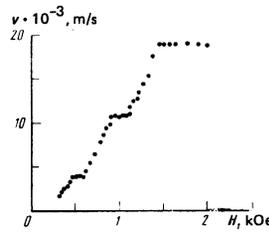
FIG. 2. Variation of the velocity of motion of a DW of intermediate type, in a mechanically polished specimen of Bi<sub>0.042</sub>Y<sub>0.958</sub>FeO<sub>3</sub>, with the amplitude of a pulsed magnetic field.
