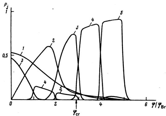
FIG. 2. Band populations vs. the angle of incidence of electrons. The numbers of the curves are the same as the numbers of the bands in Fig. 1.
