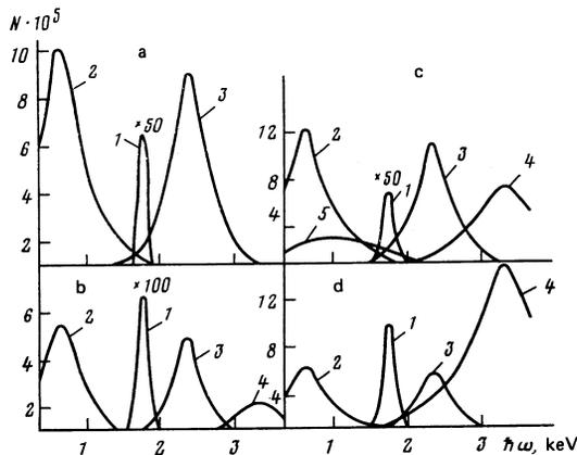
FIG. 5. Number of photons emitted, per unit length in a unit spectral interval, in the forward direction, as a result of excitation with an electron beam of  $0.3\varphi_{cr}$  divergence incident at the following angles: a) 0; b)  $0.5\varphi_{cr}$ ; c)  $0.9\varphi_{cr}$ ; d)  $1.2\varphi_{cr}$ . Transitions: 1) 2-1; 2) 3-2; 3) 3-1; 4) 4-1; 5) 4-3.
