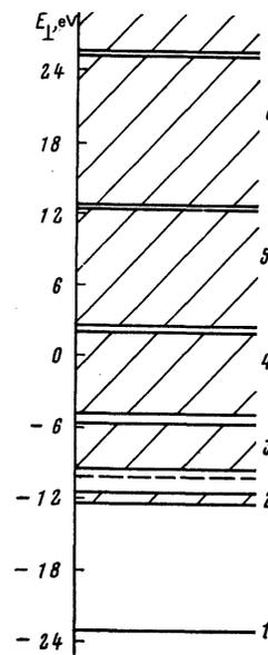
FIG. 1. Energy band structure of electrons with  $E_{k_{\perp n}} = 4$  MeV in a (110) plane of Si.
