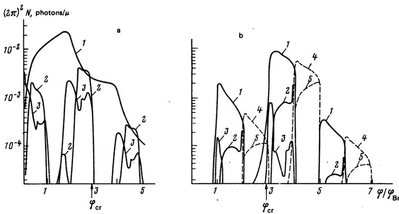
FIG. 4. Numbers of photons emitted per unit path length vs. the angle of incidence of electrons for the following transitions: a1) 2-1; a2) 3-2; a3) 3-2; b1) 4-1; b2) 4-2; b3) 4-3; b4) 5-1; b5) 5-3.
