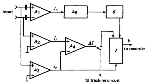
FIG. 1. Operating system of the measuring part of the apparatus;  $A_1$ —input differential amplifier;  $A_2$ ,  $A_3$ —input constant current amplifiers;  $A_4$ —differential constant current amplifier;  $A_5$ —narrow-band amplifier; 6—V9-2 phase-sensitive detector; 7—dividing unit.
