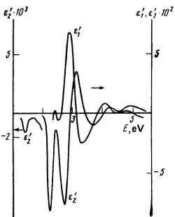
FIG. 3. The real and imaginary parts of the off-diagonal elements of the permittivity tensor for hematite.
