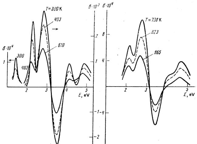
FIG. 5. The equatorial Kerr effect at different temperatures.
