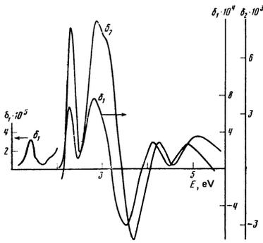
FIG. 2. The equatorial Kerr effect in hematite for two angles of incidence of the light on the specimen:  $\delta_1 - \varphi_1 = 15^\circ$ ;  $\delta_2 - \varphi_2 = 70^\circ$ .
