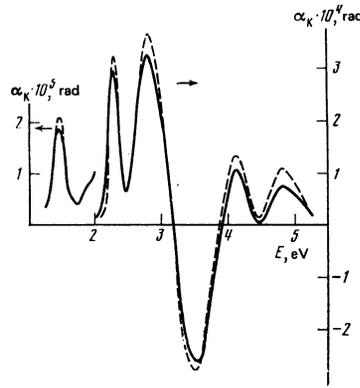
FIG. 4. The meridional Kerr effect. Solid curve, experimental; dashed curve, calculated.
