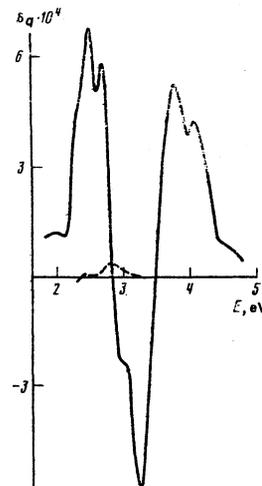
FIG. 7. The quadratic magneto-optical effect in reflected light. Solid curve—experimental, dashed curve—calculated quadratic magneto-optical effect accompanying circular magnetic birefringence.
