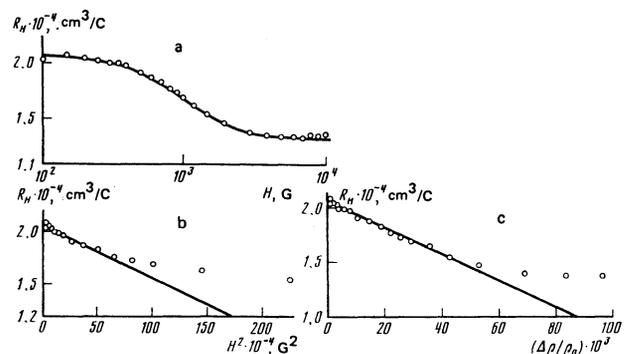
FIG. 3. Dependences of the Hall coefficient  $R_H$  for sample No. 12: a) on the magnetic field; b) on the magnetic field in the range of weak fields; c) on the magnetoresistance  $\Delta\rho/\rho_0$  in the range of weak fields.
