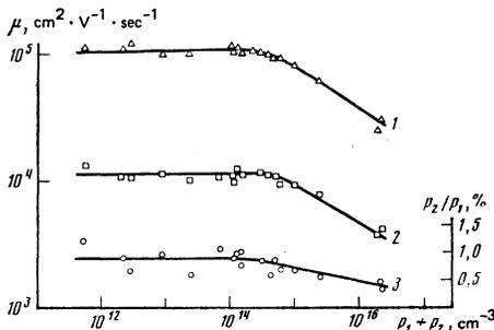
FIG. 4. Dependences of the carrier mobilities and of the ratio of the carrier densities in the light- and heavy-hole bands on the degree of doping: 1) light-hole mobility; 2) heavy-hole mobility; 3) ratio of the carrier densities in the light- and heavy-hole bands;  $p_1$  is the density of carriers in the heavy-hole band and  $p_2$  is the density in the light-hole band.
