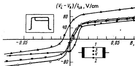
FIG. 6. Dependences of the average values of the fields between the various probes on the magnetic field, obtained for the same sample as in Fig. 5 using  $E = 113.3$  V/cm; ▲)  $(V_1 - V_2)/d_{42}$ ; ●)  $(V_1 - V_3)/d_{13}$ ; ▽)  $(V_1 - V_2)/d$ ; ○)  $(V_3 - V_4)/d_{34}$ .
