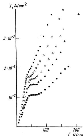
FIG. 7. Current voltage characteristics of the same sample as in Fig. 2 obtained for different pressures  $P$  along the current:  $\blacksquare$ ) 0 kG/cm<sup>2</sup>;  $\blacktriangle$ ) 1500 kG/cm<sup>2</sup>;  $\triangle$ ) 2230 kG/cm<sup>2</sup>;  $\circ$ ) 3400 kG/cm<sup>2</sup>;  $\circ$ ) 4700 kG/cm<sup>2</sup>.
