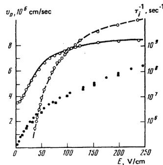
FIG. 8. Field dependences of the drift velocity (●—calculation, ■—experiment) and of the reciprocal intervalley transition time for the  $f_1$  (continuous curve) and  $f_2$  (dashed curve) phonons in *n*-type Si at 27°K.
