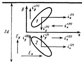
FIG. 1. Fields and partial currents in a two-valley semiconductor.
