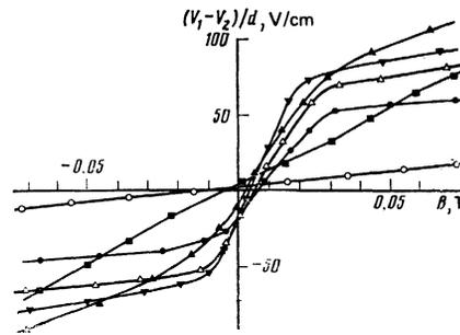
FIG. 5. Average field between the probes 1 and 2 plotted as a function of the magnetic field directed along the [001] axis, obtained for different values of  $E$ : ○) 36.2 V/cm; ●) 88.1 V/cm; △) 110 V/cm; ▽) 147 V/cm; ▲) 220 V/cm; ■) 433 V/cm.
