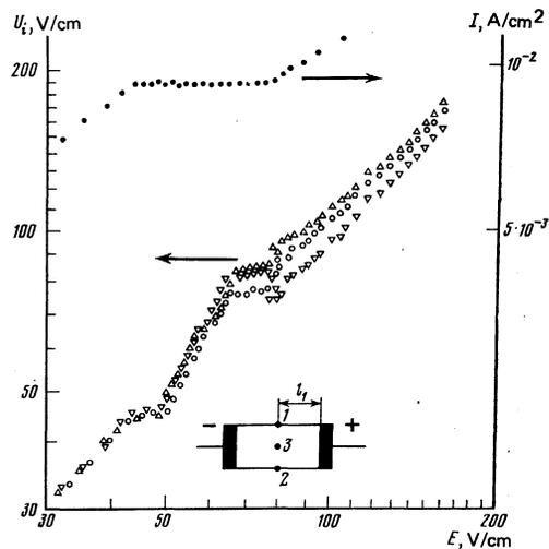
FIG. 3. Same as Fig. 2 but in the absence of a magnetic field:  $\bullet$ ) current voltage characteristic;  $\Delta$ ) probe;  $\nabla$ ) probe 2;  $\circ$ ) probe 3.
