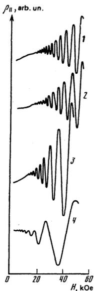
FIG. 2. Quantum oscillations of longitudinal magnetoresistivity ( $\rho_{\parallel}$ ) of sample No. 7 at various pressures (kbar): 1) 1.0; 2) 3.4; 3) 5.6; 4) 8.3.
