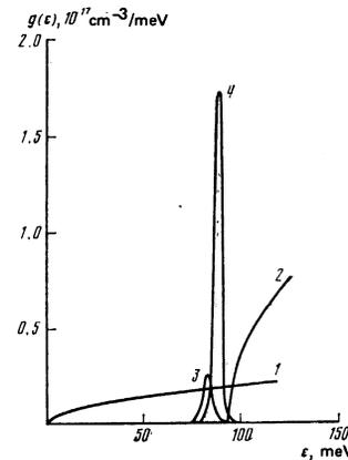
FIG. 8. State density in the impurity band of GaSb:Te: 1)  $\Gamma$  band, 2)  $L$  band (for one extremum), 3) impurity band, sample 1, 4) impurity band, sample 5.
