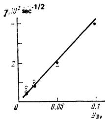
FIG. 5. Dependence of the parameter of static disordered decay on the dysprosium concentration in  $\text{La}_{1-x}\text{Nd}_x\text{Dy}_y\text{P}_5\text{O}_{14}$  crystals. ●  $x = 0.1$ ; ○  $x \approx 1$  (0.99, 0.98); △  $x = 0.5$ .
