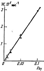
FIG. 4. Dependence of the rate of static ordered decay on the dysprosium concentration in  $\text{La}_{1-x}\text{Nd}_x\text{Dy}_y\text{P}_5\text{O}_{14}$ . ●  $x = 0.1$ ; ○  $x \approx 1$  (0.995, 0.99, 0.98); △  $x = 0.5$ .
