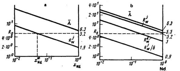
FIG. 6. Dependences of the characteristic parameters of the theory ( $\bar{\lambda}$ ) on the donor concentration in a pentaphosphate crystal: a) Nd—Nd interaction; b) Nd—Dv interaction.
