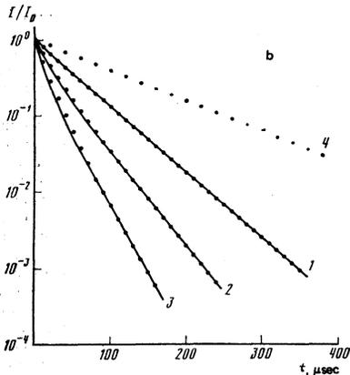
FIG. 2. Decay curves of the  ${}^4F_{3/2}$  metastable state of neodymium in a  $\text{La}_{1-x}\text{Nd}_x\text{Dy}_y\text{P}_5\text{O}_{14}$  crystal at 300 K; the points are the experimental results and the curves are theoretical. a:  $x = 0.1$ ; 1)  $y = 0.01$ , 2)  $y = 0.02$ , 3)  $y = 0.05$ , 4)  $y = 0.1$ , 5)  $y = 0$ . b: 1)  $x = 0.995$ ,  $y = 0.005$ ; 2)  $x = 0.99$ ,  $y = 0.01$ ; 3)  $x = 0.98$ ,  $y = 0.02$ ; 4)  $x = 1.0$ ,  $y = 0$ .
