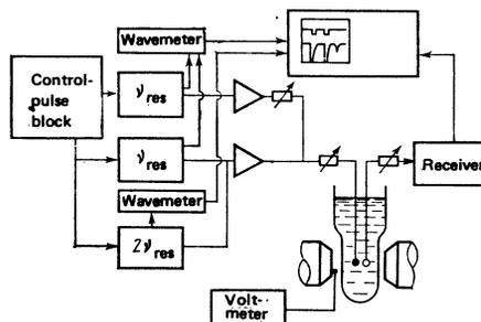
FIG. 1. Block diagram of pulsed NMR spectrometer.
