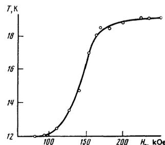
FIG. 5. Temperature recorded by thermocouple as a function of amplitude  $H_a$  of pulsed field:  $T_1 = 12\text{ K}$ .
