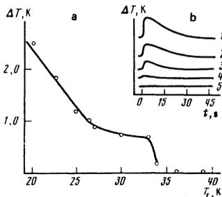
FIG. 4. a, Temperature jump recorded by thermocouple after a pulse of field  $H_a = 190\text{ kOe}$ , as a function of initial temperature  $T_1$ . b, variation of thermocouple reading with time after a pulse of field  $H_a = 190\text{ kOe}$ , for various values of  $T_1$ : 1,  $22.5\text{ K}$ ; 2,  $25\text{ K}$ ; 3,  $33\text{ K}$ ; 4,  $34\text{ K}$ ; 5,  $39\text{ K}$ .
