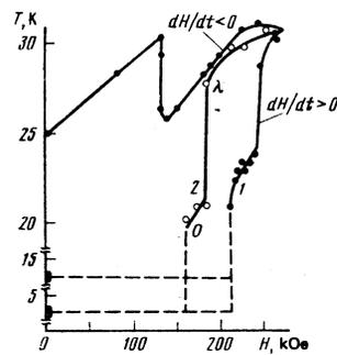
FIG. 1. Variation of values of the magnetocaloric effect with magnetic field intensity at  $T_1 = 14\text{ K}$ :  $\bullet$ ,  $H_a = 270\text{ kOe}$ ;  $\circ$ ,  $dH/dt = 0.150\text{ kOe} \leq H_a \leq 270\text{ kOe}$ .
