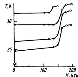
FIG. 2. Variation of values of the magnetocaloric effect with magnetic field intensity for various values of the initial temperature  $T_1$ .  $\bullet$ , antiferromagnetic phase;  $\circ$ , paramagnetic phase.
