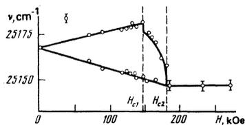
FIG. 3. Variation of splitting of the exciton line  $25\,168\text{ cm}^{-1}$  with magnetic field intensity:  $T_1 = 14\text{ K}$  ( $dH/dt = 0$ ).
