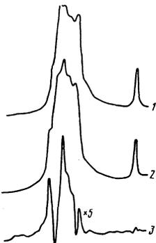
FIG. 2. ESR spectra showing  $\chi''(H) = \int (\partial\chi''/\partial H)dH$  in darkness (1) and during illumination (2). Spectrum 3 is the difference ( $\Delta\chi''$ ) between spectra 2 and 1.
