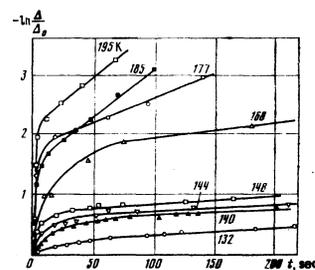
FIG. 4. Recovery of the dark ESR signal after the end of illumination:  $\Delta_0$  is the effect during illumination and  $\Delta_t$  is the effect after a time  $t$  from the end of illumination.
