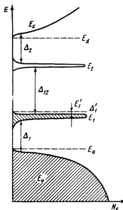
FIG. 9. Preliminary energy-level scheme of silicon:  $\Delta_1 = 0.42$ ,  $\Delta_2 = 0.43$ ,  $\Delta_{12} = 0.25$ ,  $\Delta_1' \leq 0.03 \text{ eV}$ ; in the case of germanium the corresponding values are  $\Delta_1 = 0.07$ ,  $\Delta_2 = 0.5$ ,  $\Delta_{12} = 0.18$ , and  $\Delta_1' \leq 0.05 \text{ eV}$ .
