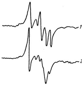
FIG. 1. ESR spectra showing the signal  $\partial\chi''/\partial H(H)$  due to dislocations in darkness (1) and the same signal in the presence of illumination (2).  $T=170^\circ\text{K}$ ,  $H_0 \parallel \langle 111 \rangle$ .
