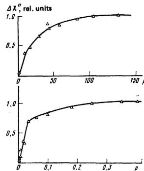
FIG. 3. Dependence of the change in the ESR signal on the optical power  $p$ ;  $\lambda = 1.3 \mu$ ; the upper curve was recorded at  $T = 200^\circ\text{K}$  and the lower at  $T = 120^\circ\text{K}$ .
