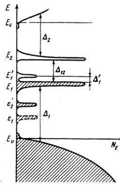
FIG. 10. Energy level scheme of the electron spectrum of dislocations.
