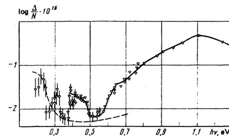
FIG. 8. Dependence of  $\log(\Delta/N)$  on the photon energy  $h\nu$ :  $\Delta$  is the change in the ESR signal due to illumination and  $N$  is the flux of the incident photons.  $T = 130^\circ\text{K}$ .
