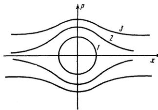
FIG. 2. Trajectory of rays in the phase plane  $(p, x)$  in the unperturbed case: 1—wave rays, 2—separatrix, 3—radiated rays.
